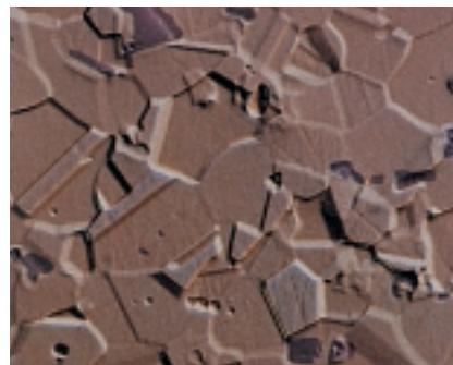
High-alloy steel, Fe-sputtered, interference contrast
