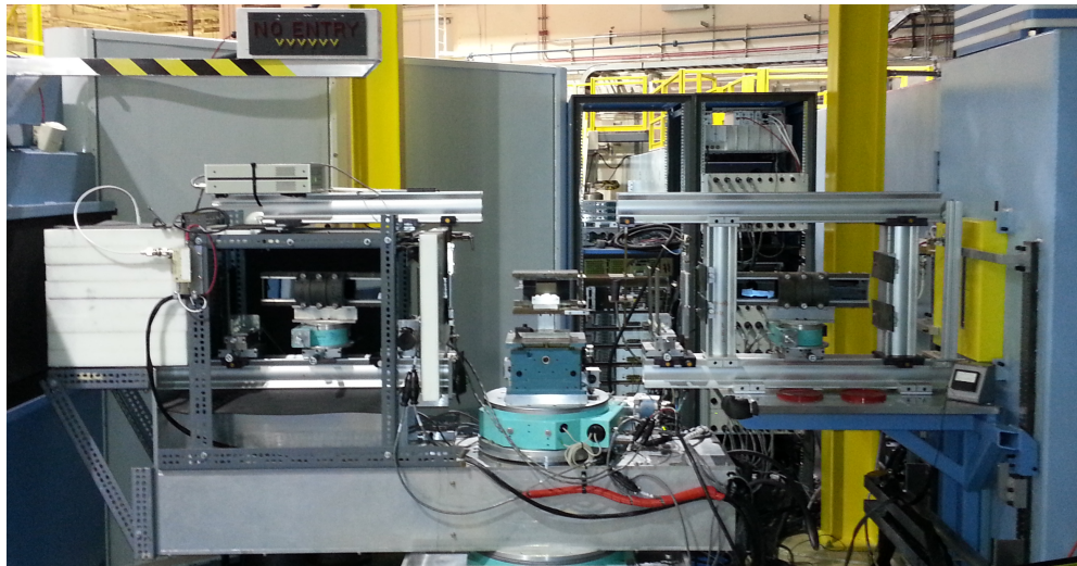
Figure 2: PBR beamline. The sample is mounted on the center goniometer, while the white detector housing is shown at far left. Polarizing supermirrors and spin flippers are visible on either side of the sample position.
