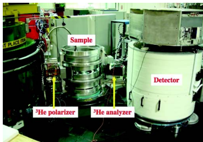
Fig. 4 The BT-7 triple-axis spectrometer with the polarized beam system installed.
