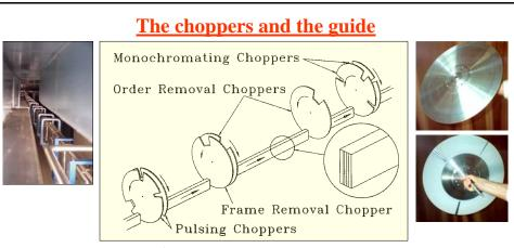
The *pulsing* and *monochromating* choppers are counter-rotating pairs, permitting a choice of pulse widths; they normally run at 20,000 rpm. The *order removal* choppers (also 20,000 rpm) remove contaminants. The *frame removal* chopper *alleviates* the problem of frame overlap. It runs at 20,000/m or 20,000(m-1)/m rpm; m is a small integer (typically m $\sim\lambda/2$ ).
