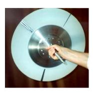
The *pulsing* and *monochromating* choppers are counter-rotating pairs, permitting a choice of pulse widths; they normally run at 20,000 rpm. The *order removal* choppers remove contaminants (also 20,000 rpm). The *frame removal* chopper *alleviates* the problem of frame overlap; it runs at 20,000/m or 20,000(m-1)/m rpm, where m is a small integer (typically  $m\sim\lambda/2$ ).
