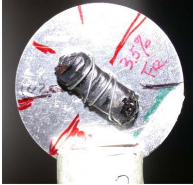
**Figure 2.** A 3.5% Fe doped  $\text{Mn}_{1-x}\text{Fe}_x\text{WO}_4$  single crystal mounted on an aluminum plate.
