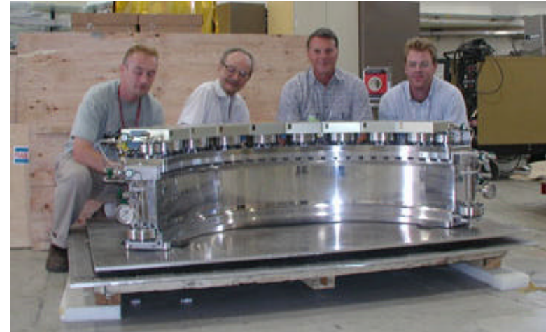
Pixelated detector covering a wide range of scattering angles (vertical & horizontal)
