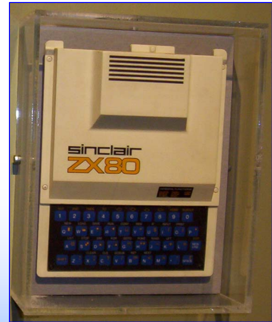
A personal computer from 1979 The Sinclair ZX80 launched the British home computer market. It was available in ready made or in kit form for under £100. The ZX80 weighs twelve ounces. It used a television for display and a cassette recorder for input. It shipped with 1K static RAM, expandable to 16K
