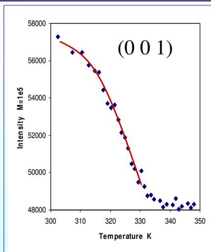
$I \sim (1-T/T_c)^{2\beta}$ , the fitted parameters  $T_c = 330\text{K}$  and  $\beta = 0.333$
