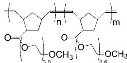
**Figure 1.** Chemical structure of block copolymer  $(\text{EG}_3\text{NB})_{79}$ – $(\text{EG}_{6,6}\text{NB})_{67}$ .
