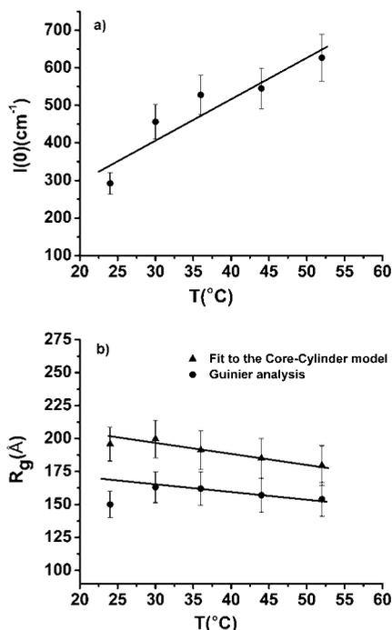
**Figure 3.** Results of the Guinier analysis of the SANS data of the block copolymers in 2.0 wt.% D<sub>2</sub>O. Key: (a)  $I(0)$  as a function of temperature; (b)  $R_g$  as a function of temperature. The radius of the core of the micelles has a polydispersity of 0.15 based on the modeling of the SANS data, which defined the error bars of the  $R_g$  shown in the figure. The solid lines in Figure 3 are guides to the eye.
