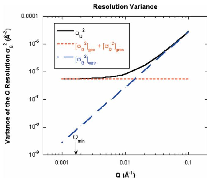
**Figure 1** Variation of  $\sigma_Q^2$  with  $Q$  plotted on a log–log scale. The two main contributions (geometry and wavelength spread) are added in quadrature. Gravity effects are small for the wavelength considered here ( $\lambda = 6 \text{ \AA}$ ).
