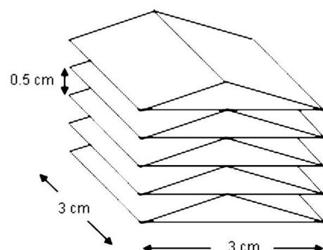
**Figure 6** Representation of the prism cassette containing a row of five MgF<sub>2</sub> prisms.
