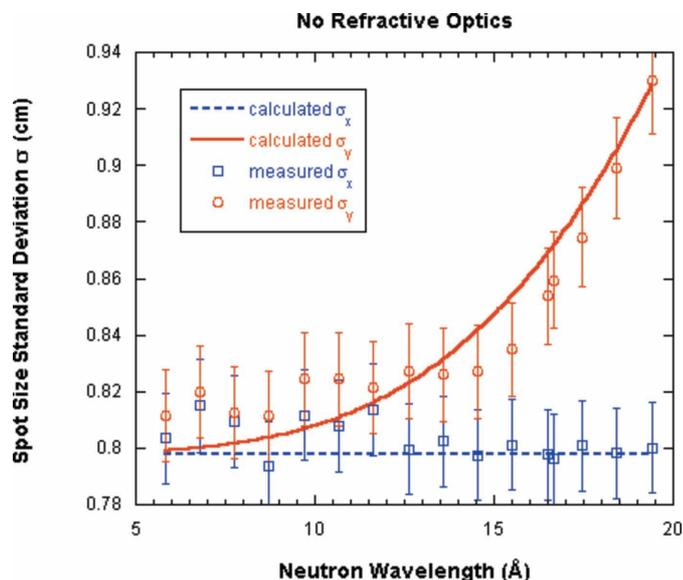
**Figure 2** Variation of the measured and calculated neutron spot-size standard deviations  $\sigma_x$  and  $\sigma_y$  with increasing wavelength. Statistical error bars (obtained from the fits) have been included.
