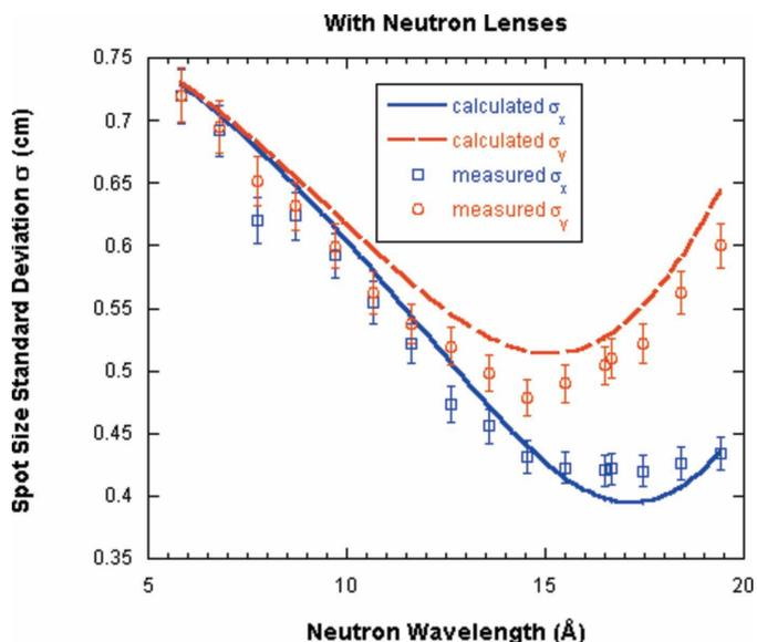
**Figure 4** Variation of the spot-size standard deviation with wavelength in the horizontal and vertical directions. The calculated trends agree with the measured ones. Statistical error bars have been included.
