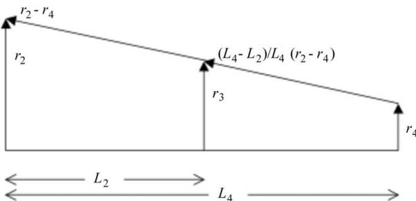
**Figure 9** A schematic diagram indicating the construction of the vector  $\mathbf{r}_3$  on the detector plane of the general trajectory that passes through the uncorrelated points given by the vectors  $\mathbf{r}_2$  on the lens plane and  $\mathbf{r}_4$  on the image plane. The detector plane and the image plane are at distances  $L_2$  and  $L_4$ , respectively, from the lens plane.
