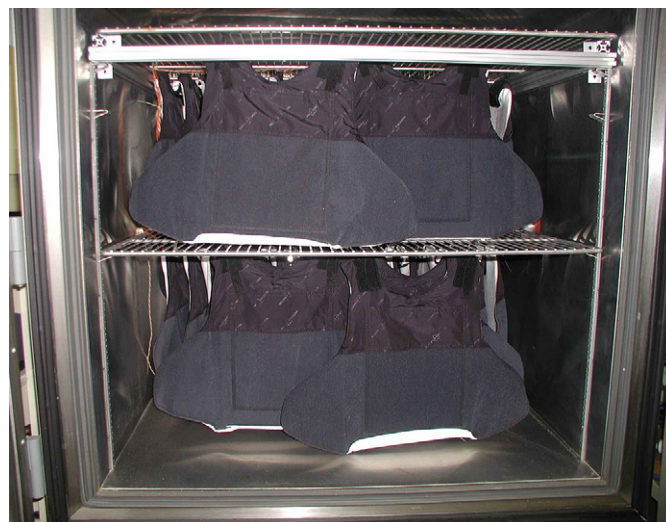
Fig. 1. Front panels of vests hanging in environmental chamber.
