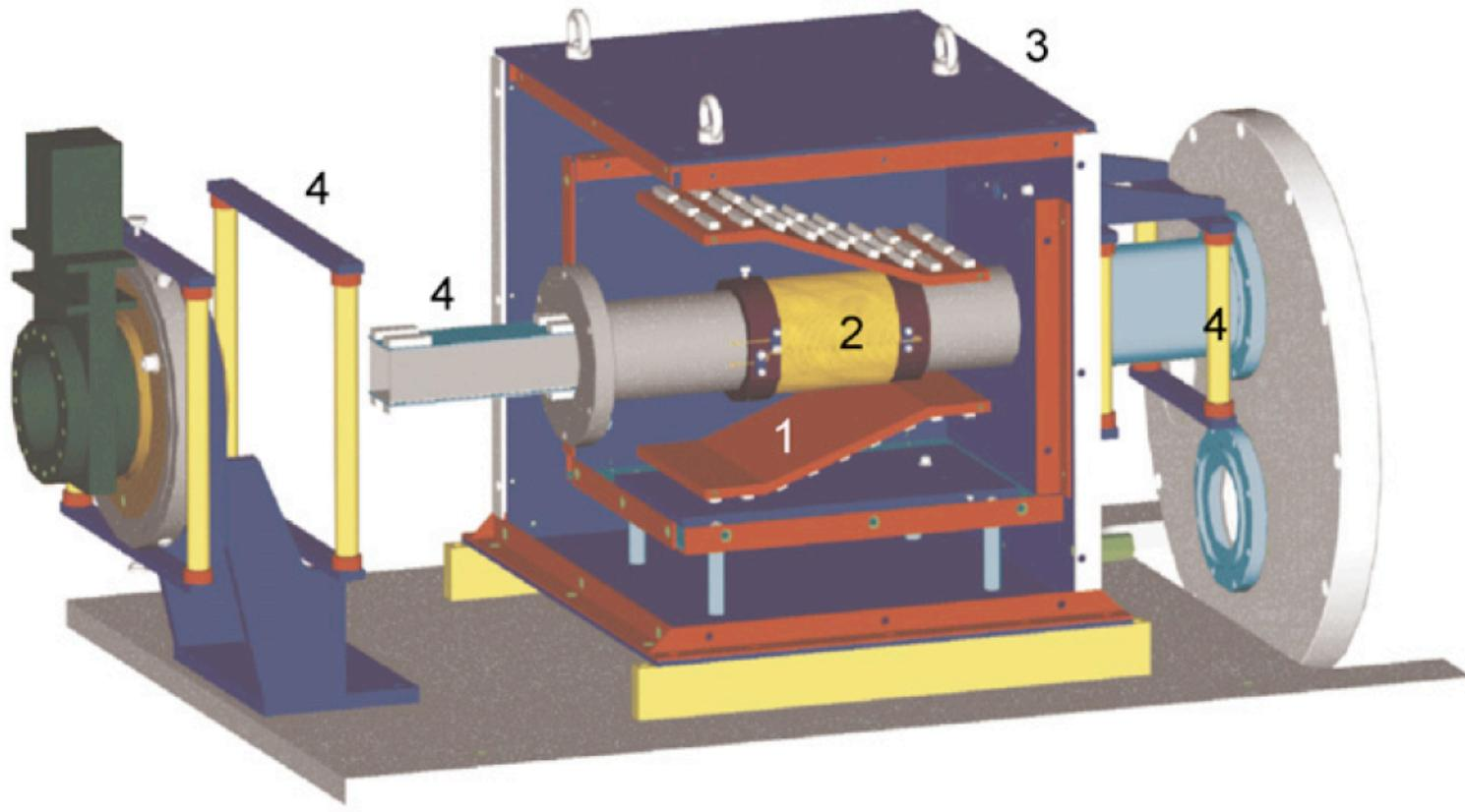
Fig. 3. Schematic drawing of the spin flipper setup with (1) the gradient field, (2) the radio-frequency solenoid, (3) the magnetic shielding box and (4) the magnetic guiding field.
