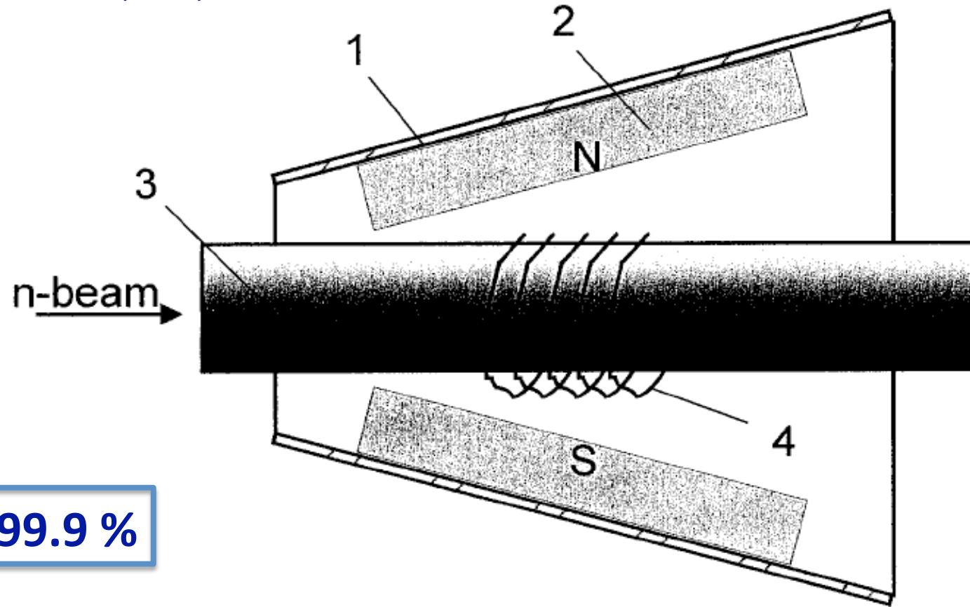
Fig. 3. RF gradient spin flipper. (1) Iron yoke (length 21 cm, width 22 cm/37 cm at left/right side); (2) Ferrite permanent magnets  $20 \times 10 \times 2$  cm<sup>3</sup>; (3) Beam tube (ceramic,  $\varnothing$  11 cm); (4) RF coil.
