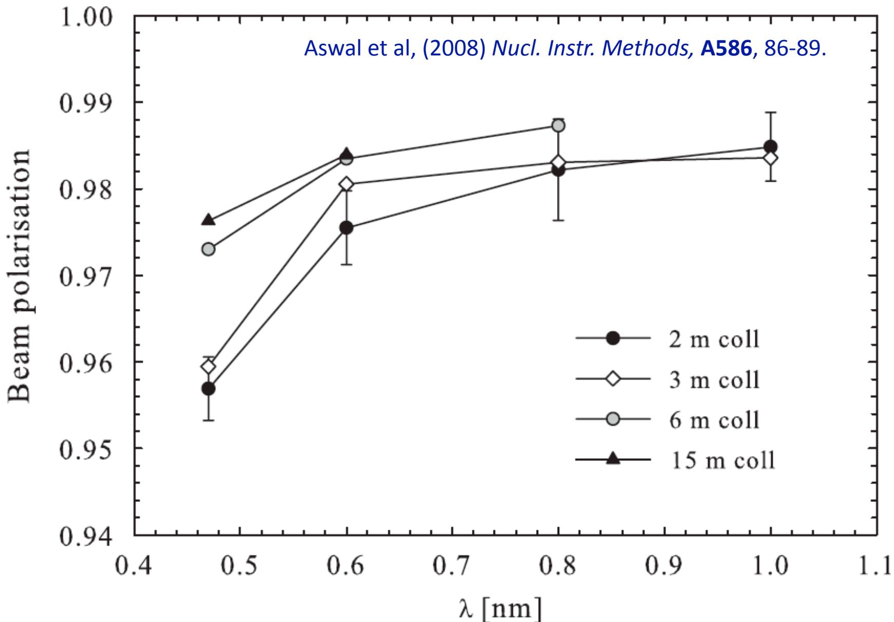
Fig. 4. Polarisation of the neutron beam at SANS-I at SINQ for different collimation lengths. For clarity the measurement error is shown for one
