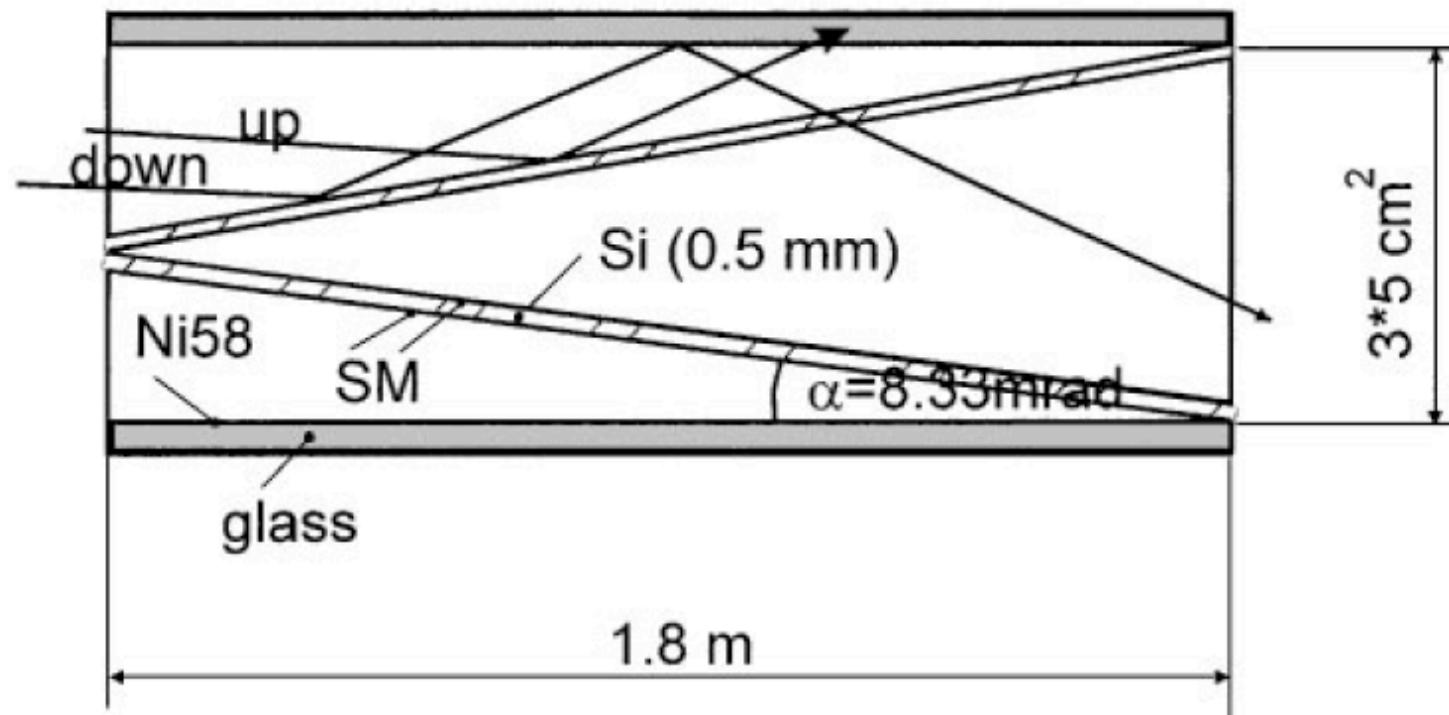
Fig. 2. Transmission polarizer (top view). Si-wavers with super-mirrors on both sides are arranged in a V-shape inside a neutron guide. Spin-down neutrons are transmitted, spin-up neutrons are absorbed in the glass walls.
