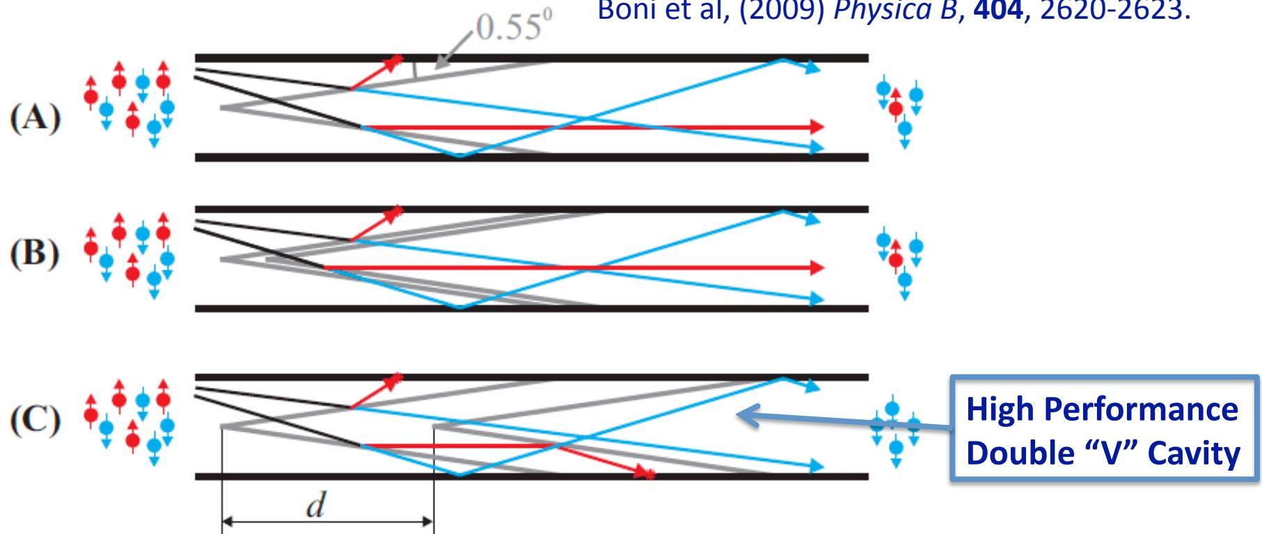
Fig. 4. Top view of polarizing cavities. If a single V-cavity is used (A), there is a possibility that neutrons with the up-polarization are transmitted. If the two Vs are displaced by a significant distance  $d$  (C), the wrongly polarized neutrons are removed and the polarization of the transmitted beam is increased. If the Vs are too close (B),  $P$  does not improve.
