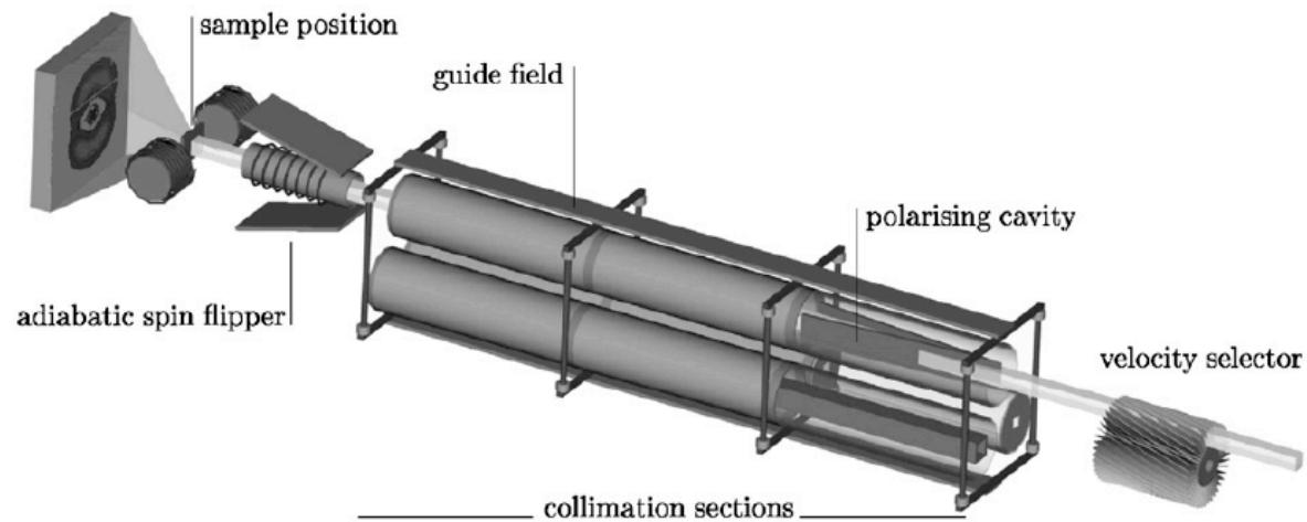
Fig. 1. Sketch of the polarisation option at SANS-I. The polarising cavity is located inside a neutron guide (not shown) within the first exchangeable segment of the collimator.
