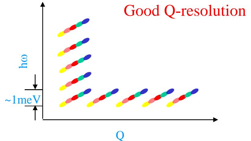
Probes scattering events at different energy and momentum transfers simultaneously
