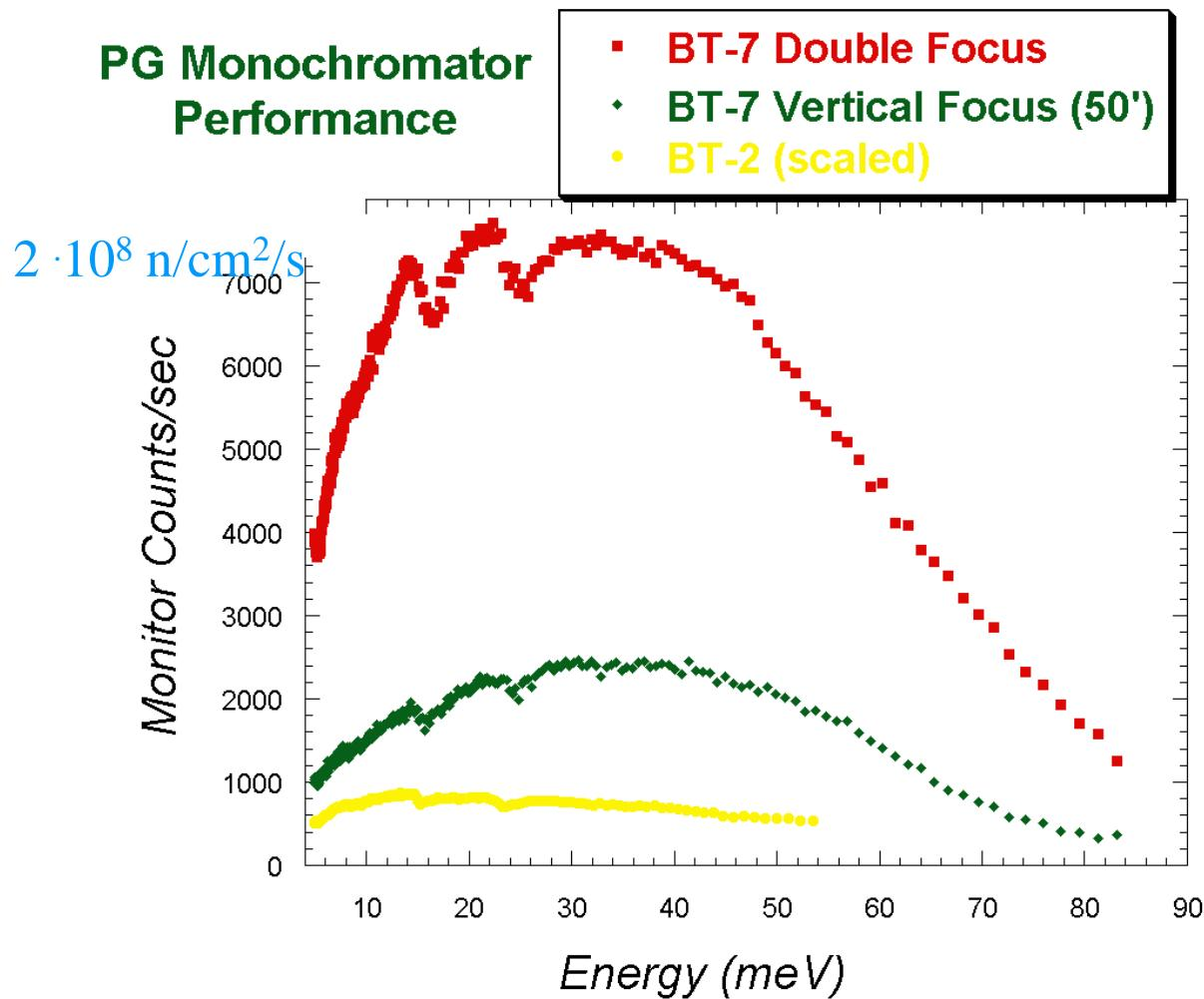
With vertical focusing, gain of 2.3 over BT-2/9 at 14.7 meV; gain of 3.5 at 40 meV.
