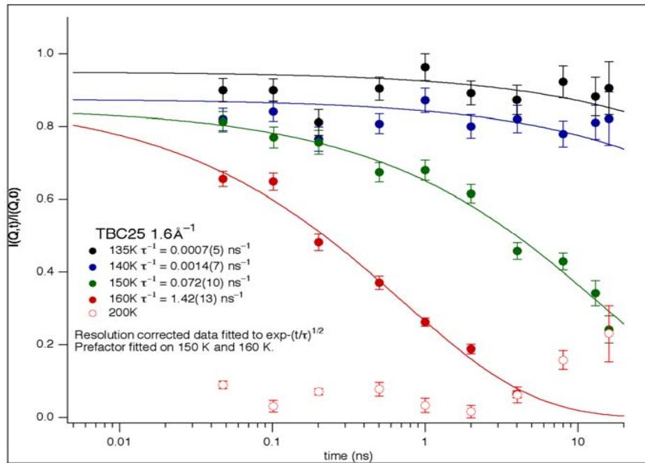
Intermediate scattering function of Toluene with 25% Benzyl Chloride at the structure factor peak above the glass temperature. The data are fitted with a stretched exponential using the usual exponent of 1/2.
