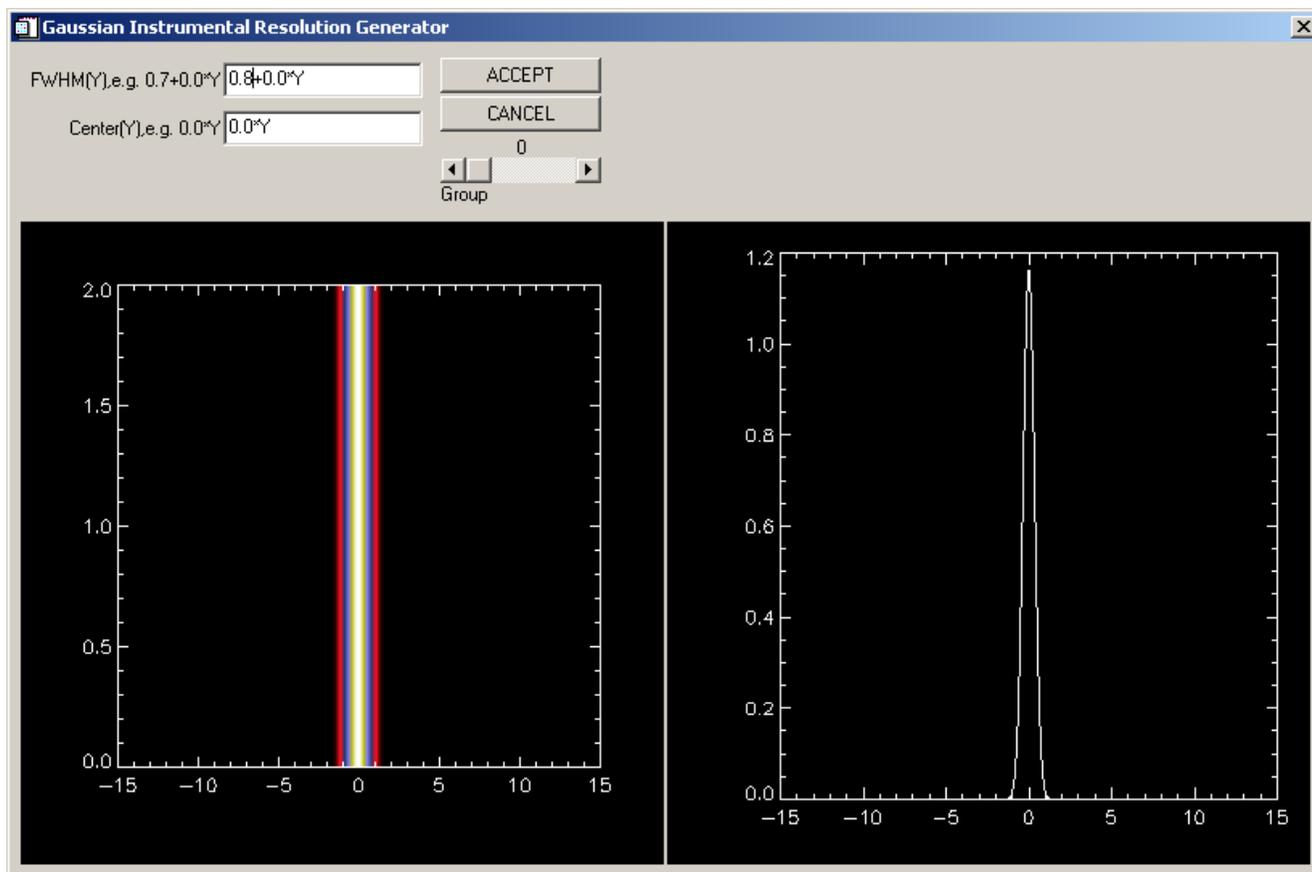
Fig. 5 Gaussian instrumental resolution function generator application.
