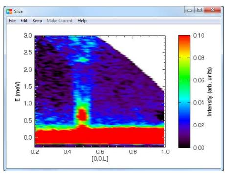
7. Choose the cutting axis and thickness over the other two axes, and press **Plot Cut** to plot the cut.
