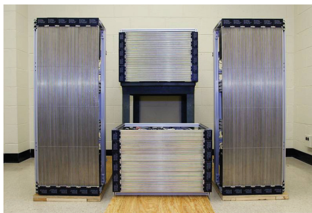
FIGURE 2: Assembled “8-pack” ^3\text{He} proportional counter arrays for vSANS.
