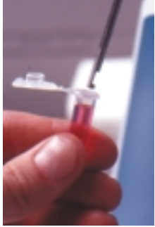
The microprobe can measure sample volumes as low as 120 µL.
