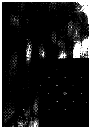
Fig. 1. Electron micrograph showing one family of twin boundaries in our \text{YBa}_2\text{Cu}_3\text{O}_7 crystal. The inset is a selected-area diffraction pattern (20- \mu\text{m} aperture) with the electron beam in the [001] direction, showing the orthorhombic splitting of the reflections.
