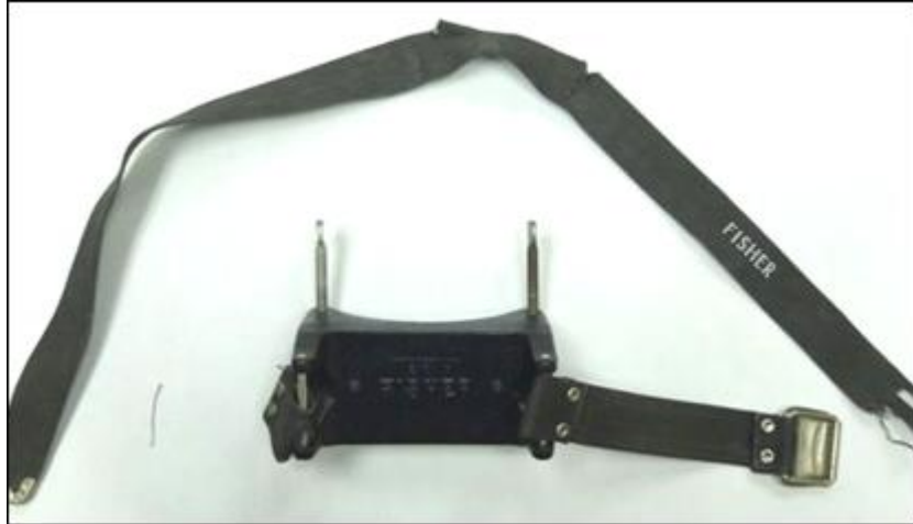
Figure 3: Image of Fisher brand wall mounted compressed gas cylinder bracket used at NIST. Note the tears in the cotton strap and torn cotton webbing in the buckle location. These tears were intentionally produced by staff to show how frail the cotton strap had become.
