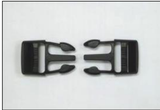
Figure 2: Image of a defective (left) and non-defective (right) buckle. The defective buckle is angled inward which results in minimal force being required to cause the snap clip to disconnect.
