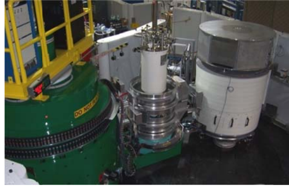
Fig. 4. Photograph of the thermal triple axis instrument at BT-7 in operation. The electronics for the front portion of the instrument (through the sample position) resides on top of the (green) monochromator drum, while the sample environment system is the top-loading \text{He}^3 system with a base temperature of 300 mK. The sample is surrounded by the sample enclosure to adsorb scattered neutrons and reduce ambient instrumental background. The analyzer system is below 17^\circ so that the beam stop is in the up position. Two PG filters and an x-y slit system are on the x-rail in front of the analyzer system. The electronics for the analyzer system resides on top of the analyzer.
