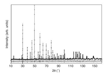
Fig. 3. Observed, calculated, and difference neutron diffraction profiles for the pyrochlore  $0.4400:0.2700:0.2900 \text{ Bi}_2\text{O}_3:\text{Fe}_2\text{O}_3:\text{Nb}_2\text{O}_5$  at 10 K. Tick marks indicate allowed reflection positions.
