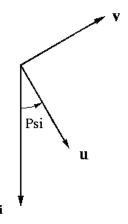
(**ux**, **uy**, **uz**) and (**vx**, **vy**, **vz**) specifies the two *reciprocal* crystal axes.  $u \times v$  should point to the vertically *upward* direction. **Psi** is the angle between u and ki, and is positive if ki  $\times$  u is pointing to the vertically upward direction. For DCS file type, it should be the same as DCS A2 angle if A2 is set to 0° when ki is parallel to u. For *diffuse scattering*, Psi is the angle for the first file.
