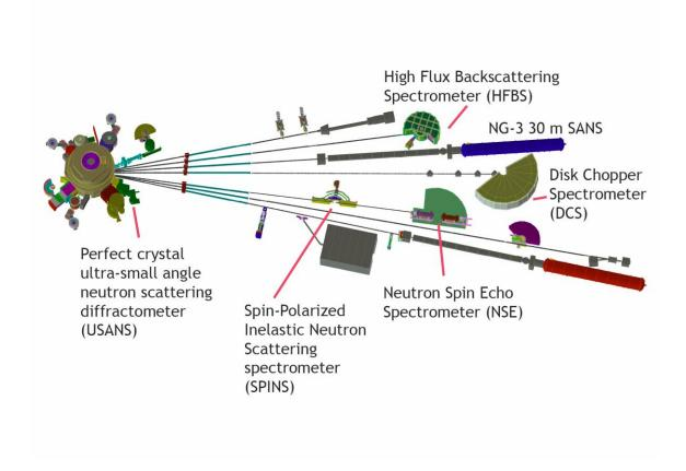
Schematic array in 2002 of the instrumentation suite at the NCNR. The six cold neutron instruments which comprised the NSF/NIST Center for High-Resolution Neutron Scattering (CHRNS) at that time are pointed out.
