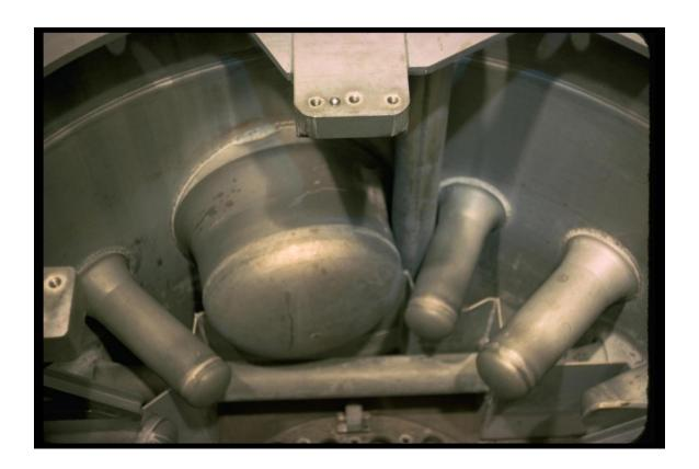
The core of the NBS reactor showing the large cold source "thimble" which was the key component of the nation's first cold neutron research facility. This picture and several others in this history are from a collection of early photos of the NMSR and its staff put together by Jim Torrance, long-time Deputy Chief of Reactor Operations.
