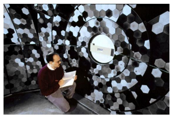
NCNR's Dan Neumann checks the large array of single crystal silicon wafers that forms the focusing analyzer of the High Flux Backscattering Spectrometer he helped design.
