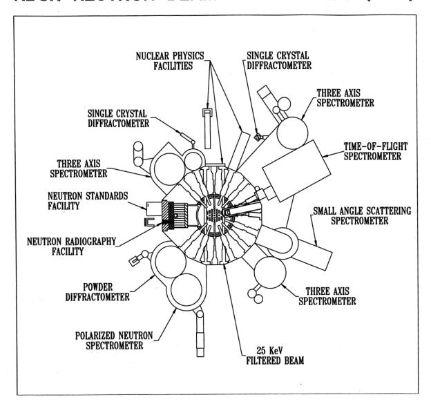
By 1975 NBS and its collaborators had developed an array of neutron scattering and other neutron beam instruments at the NBSR. A plan view of this instrument suite is shown above.
