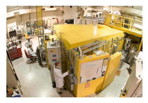
NCNR's David Jacobson stands before the Neutron Imaging Facility that has played a unique role in revealing the flow of product water during the operation of fuel cells being developed by the automotive industry for alternative vehicles. NCNR's Dan Hussey (seated) and Eli Baltic are at the controls at the left. This facility was developed in a partnership between NIST and GM, and is available for use by other U.S. researchers.
