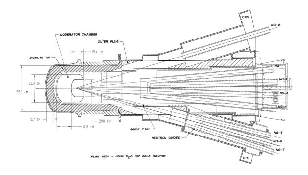
Plan view of the original large  $D_2O$  ice cold neutron source at the NBSR. Also shown emanating to the right is the network of seven guide tubes, which carried cold neutrons into the guide hall.
