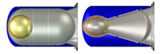
Schematic views of the hydrogen moderator cold neutron sources, which replaced the original D<sub>2</sub>O ice moderator. The original hydrogen source installed in 1995 increased cold neutron intensities by a factor of six. The second improved source (right) doubled available intensities in 2003.
