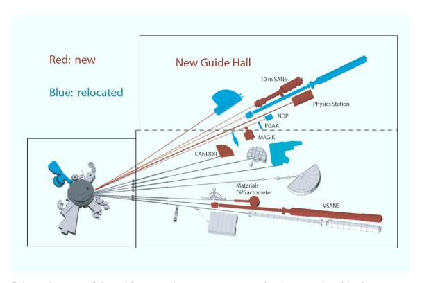
Schematic array of the cold neutron instruments expected to be operational in the expanded NCNR guide hall at the end of 2014.
