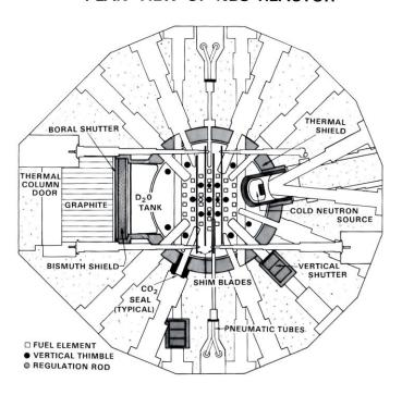
A plan view of the NBSR showing the reactor core, the large radial beams, and the location of the future large cold neutron source.
